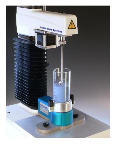
For complete testing transformation, attach a Powder Flow Analyser and you can measure the flow properties of powders. For bakery research, a Dough Inflation System allows pressure information to indicate the bi-axial extensional properties of dough.
